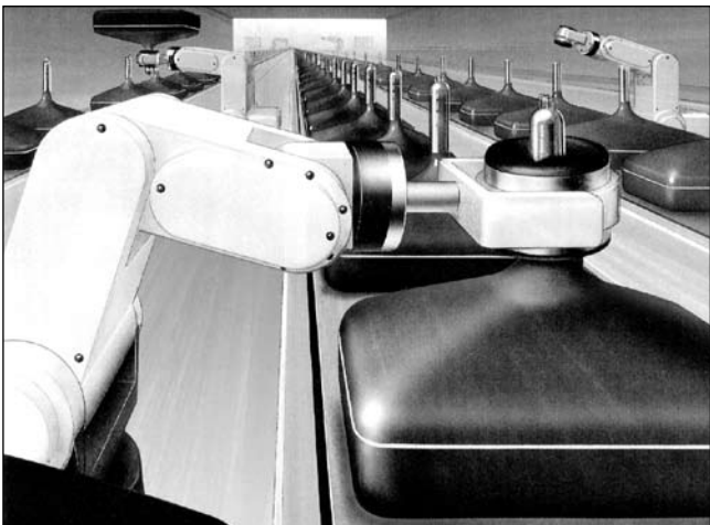
Gripping and carrying inverted TV tubes
