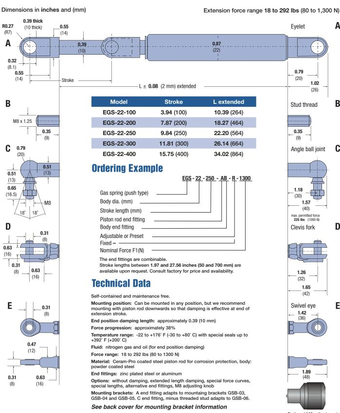
Optional M8 adjustment knob for adjusting gas pressure on adjustable models only
