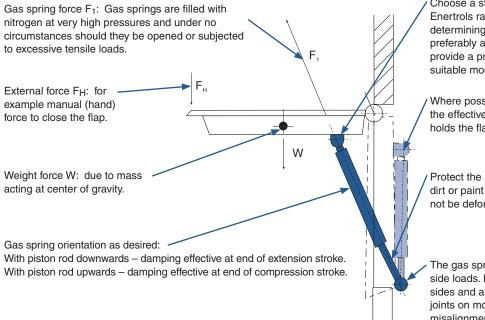
Choose a standard available gas spring from the Enertrols range featured in this catalog before determining the mounting position coordinates, or preferably allow Enertrols to do the calculations and provide a printout suggesting the most suitable model and mounting positions.
